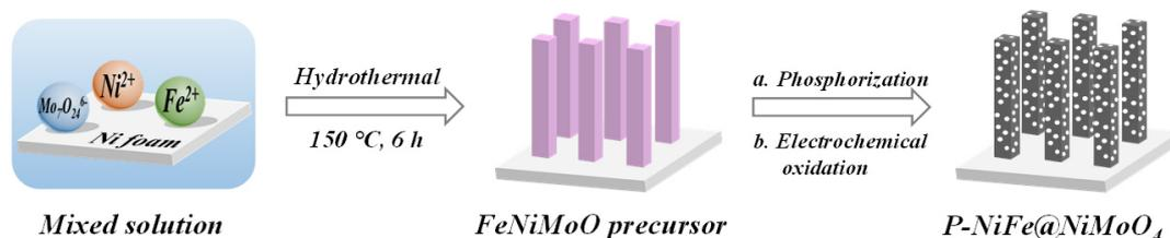
Scheme 1. Schematic of P-NiFe@NiMoO<sub>4</sub> electrode synthesis.
