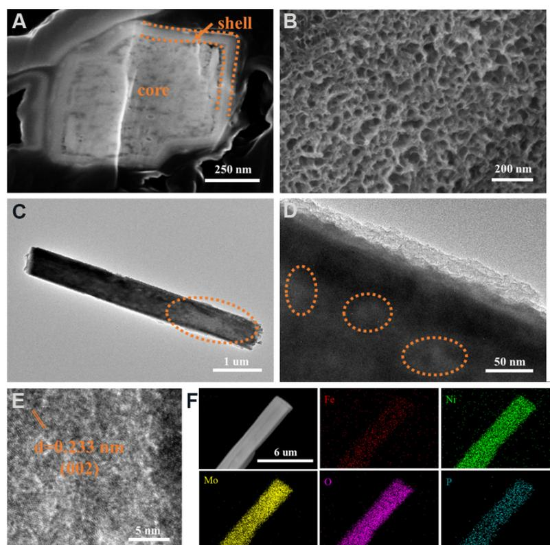
**Figure 1.** Scanning electron microscopy images of (A) a cross section of P-FeNiMoO and (B) P-NiFe@NiMoO<sub>4</sub> electrode. (C-E) Transmission electron microscopy and high-resolution transmission electron microscopy images of P-NiFe@NiMoO<sub>4</sub> scraped from nickel foam. (F) Elemental mapping images of P-NiFe@NiMoO<sub>4</sub>.
