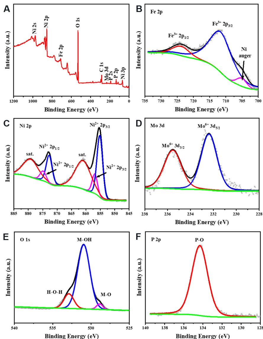
**Figure 2.** (A) X-ray photoelectron spectroscopy survey and high-resolution spectra of (B) Fe 2p, (C) Ni 2p, (D) Mo 3d, (E) O 1s and (F) P 2p for P-NiFe@NiMoO<sub>4</sub> electrode.
