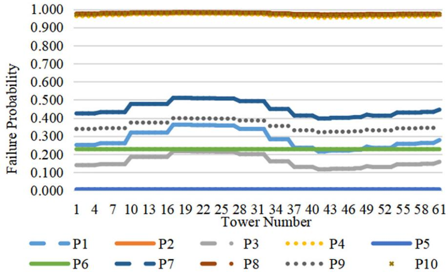
Figure 3. Damage probability of THJ line in 10 cases.
