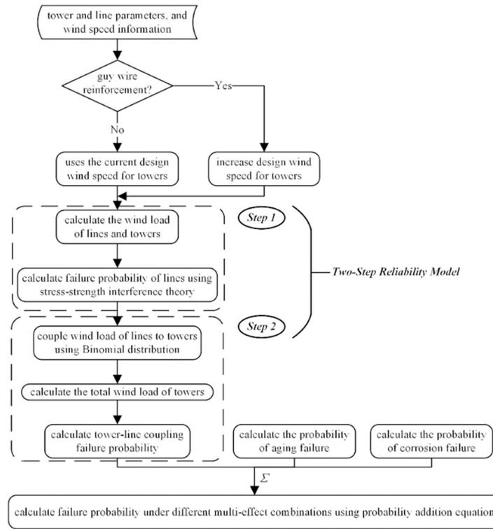
**Figure 1.** The structure diagram of damage prediction method considering multi-effect.
