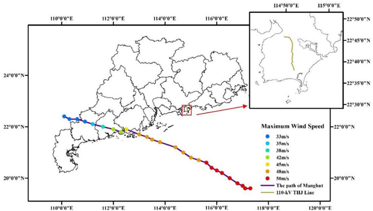
**Figure 2.** The track of strong typhoon "Mangkhut" and distribution of THJ line.
