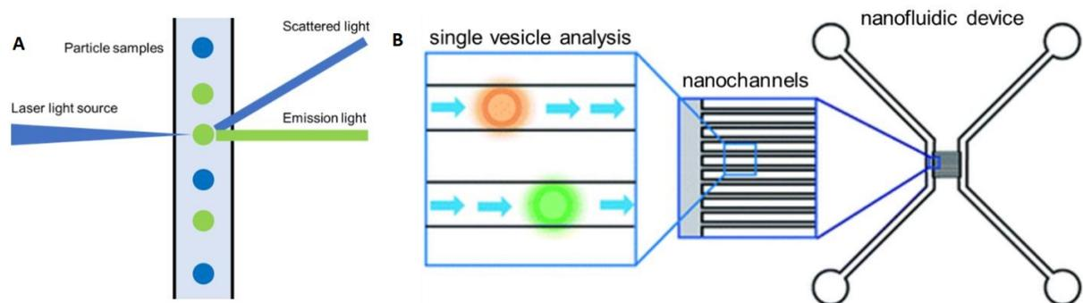
**Figure 8.** (A) The principle of flow cytometry. (B) A flow cytometry platform designed by Friedrich *et al.*<sup>[164]</sup> The nanofluidic device contained 100 nanochannels with a width of 300 nm and the dye-labeled EVs could be sensed and recorded by a fluorescent microscope (reproduced from<sup>[164]</sup>).
