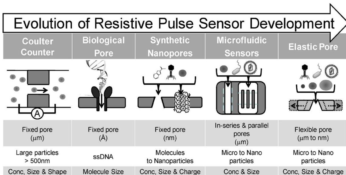
**Figure 9.** The evolution of resistive pulse sensing (RPS) from fixed pore with micro-scale to flexible pore with micro- to nano-scale sizes. RPS can also be applicable as a Coulter counter for EV analysis with the proper sized pore (reproduced from<sup>[171]</sup>).
