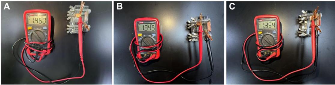
**Supplementary Figure 8.** Photographic images of the open circuit voltage for (A) Co-N<sub>4</sub>Cl-C-, (B) Co-N<sub>4</sub>-C-, and (C) Pt/C-based SWZABs.
