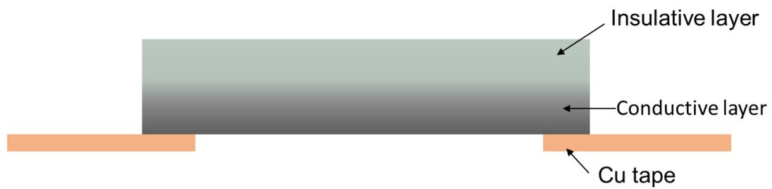
Figure S8. Schematic illustration of the electric measurement of the LME composite by contacting the Cu taper with the bottom conductive layer.
