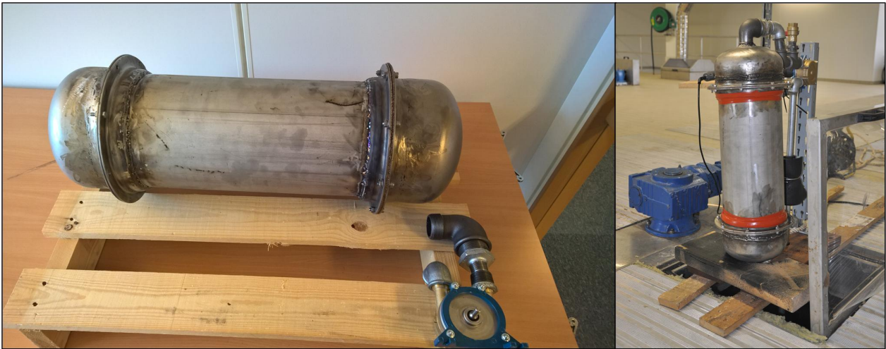
Supplementary Figure 1. Pictures of the sampling device designed and used within this study (A) and operational at GR-STP raw water inlet (B).
