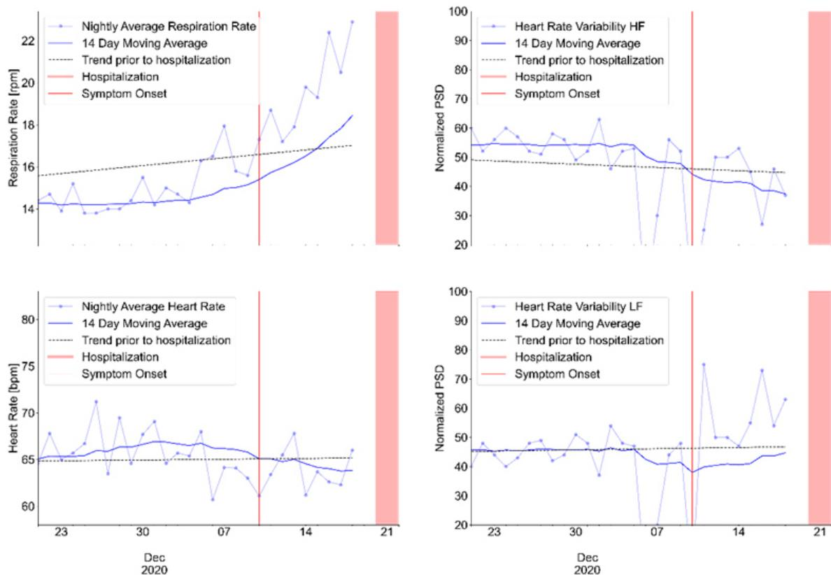
**Figure 4.** Evolution of sensor signals from an EMFIT QS bed sensor device indicating changes in respiration rate (respiration cycles/min), heart rate (beats/min), high frequency (HF), and low frequency (LF) heart rate variability (HRV-HF refers to the normalized power spectral density between 0.04 and 0.15 Hz; conversely, HRV-LF refers to the same between 0.15 and 0.4 Hz).
