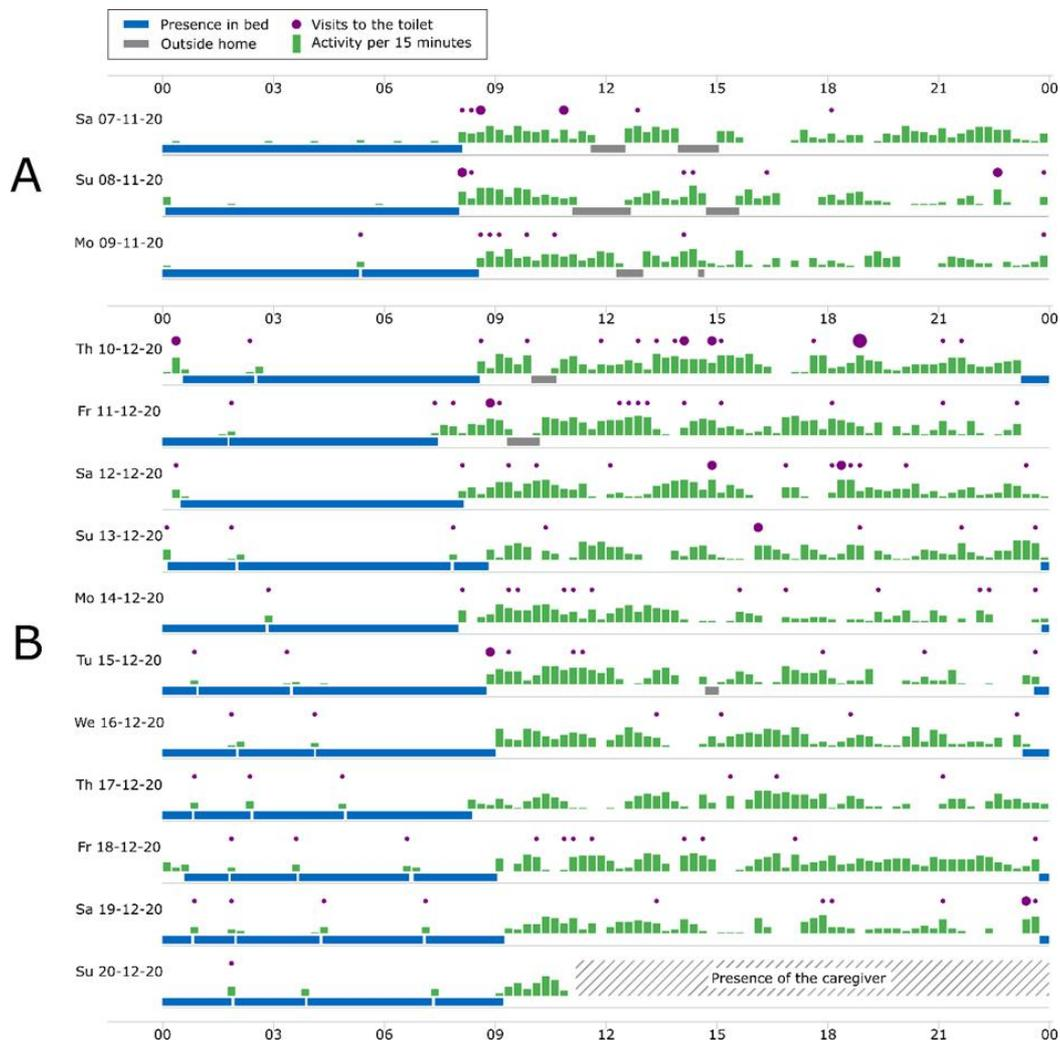
**Figure 1.** Dashboard for caregivers with visualization of daily activities (normalized units) based on sensor data from passive infrared (PIR) motion sensors in each room of the home which is regularly used, a door sensor at the entry door of the home, and an EMFIT QS bed sensor. The figure shows three representative days for the situation in November before COVID-19 (A) and the days from diagnosis to hospitalization 10 days later (B).
