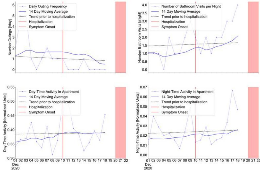
**Figure 3.** Evolution of sensor signals from a combined ambient passive infrared motion sensor system to monitor outings (leaving home), daytime and nighttime activity (normalized units), and bathroom visits at night.
