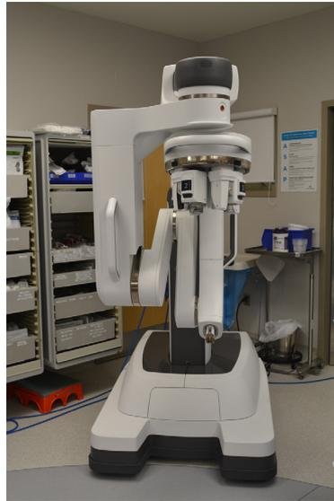
**Figure 4.** Single port robotic platform
