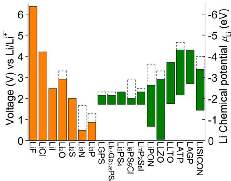
**Figure 10.** Calculated electrochemical stability windows for a variety of solid electrolytes. The dashed lines mark the oxidation potentials to fully delithiate the material. Reproduced with permission<sup>[106]</sup> (Copyright 2015, American Chemical Society).
