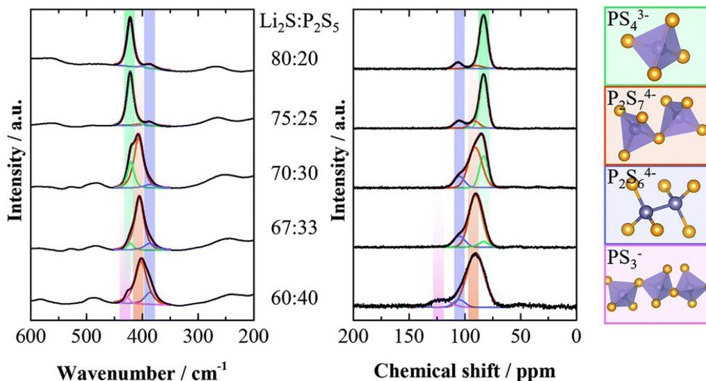
**Figure 4.** Raman and <sup>31</sup>P magic angle spinning-nuclear magnetic resonance (MAS-NMR) spectra of xLi<sub>2</sub>S-(100-x)P<sub>2</sub>S<sub>5</sub> glasses with different Li<sub>2</sub>S contents. Reproduced with permission<sup>[62]</sup> (Copyright 2017, Royal Society of Chemistry).
