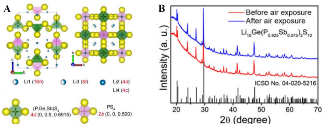
**Figure 11.** (A) Crystal structure of  $\text{Li}_{10}\text{Ge}(\text{P}_{0.925}\text{Sb}_{0.075})_2\text{S}_{12}$ . (B) XRD patterns of  $\text{Li}_{10}\text{Ge}(\text{P}_{0.925}\text{Sb}_{0.075})_2\text{S}_{12}$  sample before and after air exposure. Reproduced with permission<sup>[49]</sup> (Copyright 2020, American Chemical Society). XRD: X-ray diffraction.
