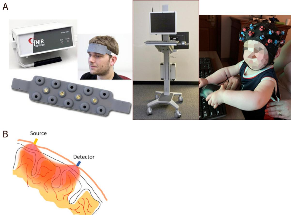
**Figure 3.** Left: the NIRS apparatus; Middle: the data-capturing device; Right: NIRS cap (NIRx NIRSport2 Wireless system) containing sources (red marks) and detectors (blue marks) are placed on the participants' head (A); light enters the tissue from location of source and backscattered photons are detected at the detector site (B). The detected light intensity carries information about changes in oxy-hemoglobin and deoxy-hemoglobin. NIRS: near infrared spectroscopy
