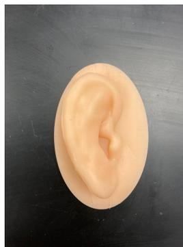
**Figure 8.** In-house 3D-printed auricular hematoma simulator<sup>[28]</sup>.
