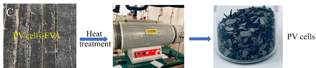
Recovery of PV cells
