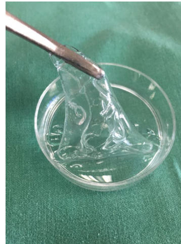
Figure 3: The gross view of cross-linked hyaluronic acid using BDDE at the concentration of 0.8%
