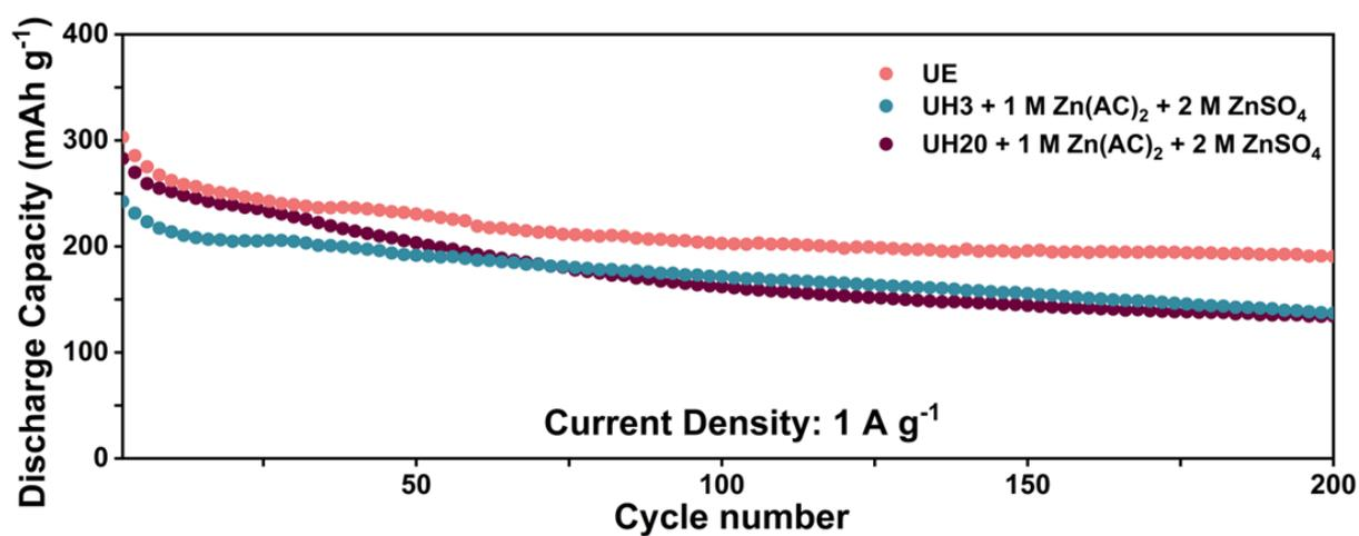
**Figure S12** The cycling performance of Zn//I<sub>2</sub>@ AC batteries with different urea ratios at a current density of 1 A g<sup>-1</sup>.
