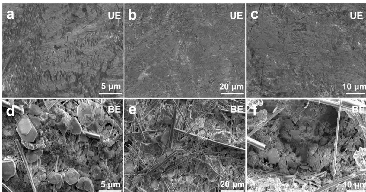
**Figure S5** SEM of Zn anode after 50 cycles of various electrolytes.
