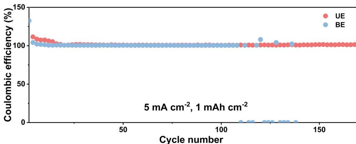
Figure S7 Coulombic efficiency of Zn//Cu cells in UE and BE.
