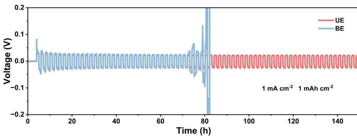
**Figure S6** Voltage responses of Zn//Zn symmetric cells in UE and BE with the areal capacity of  $1 \text{ mAh cm}^{-2}$  (current density of  $1 \text{ mA cm}^{-2}$ ) for 150 h.
