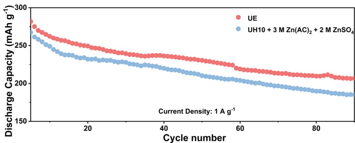
**Figure S13** Cycling performance of Zn//I<sub>2</sub>@ AC batteries in different concentrated electrolytes at 1 A g<sup>-1</sup>.
