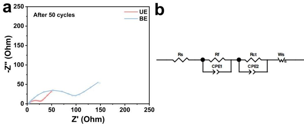
**Figure S14** The (a) fitted impedance diagrams and (b) equivalent circuit diagrams of UE and BE.
