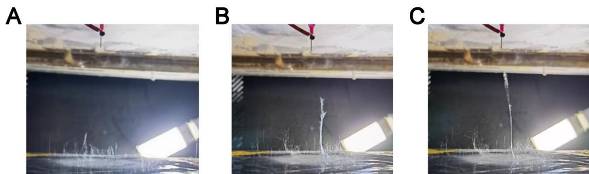
Supplementary Figure 6. Electrospinning process of the PVDF-HFP/[EMIM][TFSI] iontronic nanofibers with iontronic liquid weight rate of 2:1.
