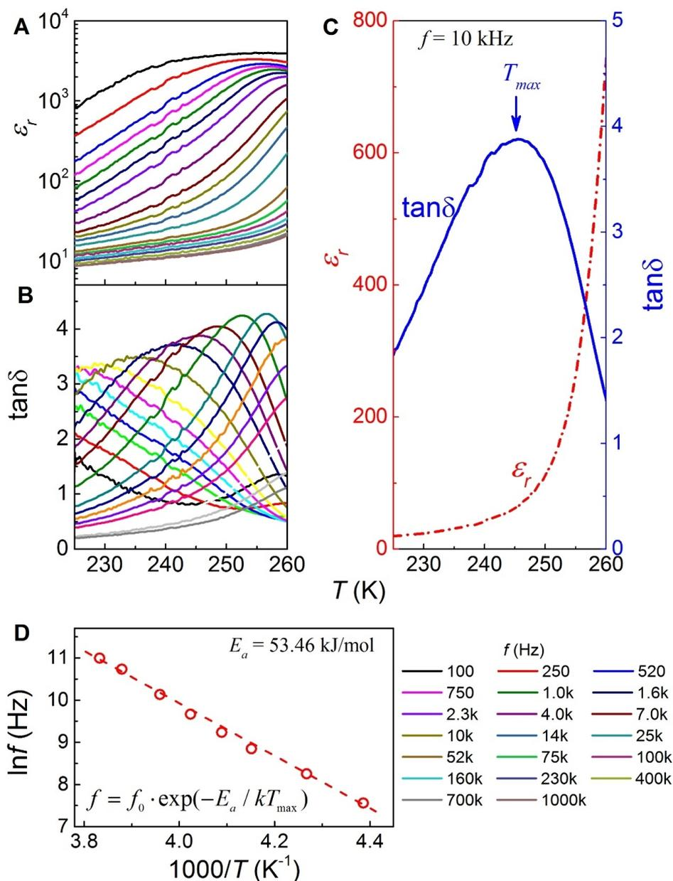
**Figure 5.** (A) and (B) measured dielectric real part  $\epsilon_r$  and loss  $\tan\delta$  at several frequencies as a function of  $T$  for the as-prepared wet sample ( $f_w = 0.483$ ) in the warming sequence from 200 K. For a clearer illustration, the measured  $\epsilon_r(T)$  and  $\tan\delta(T)$  data at  $f = 10$  kHz are presented in (C). (D) Evaluated  $T_{max}$  vs.  $f$  relationship from which the thermal activation energy  $E_a$  is evaluated via the Arrhenius law.
