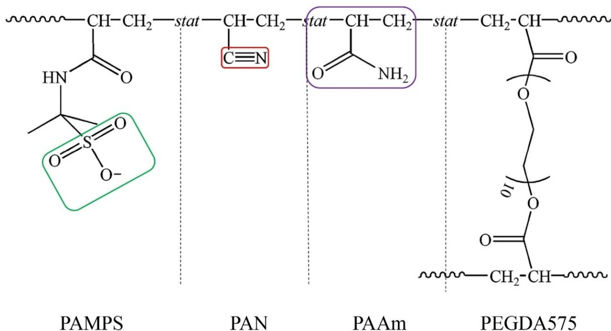
**Figure 2.** Schematic of the molecular structure and the basic structural units of the PAN-based hydrogel, where PAMPS, PAN and PAAm and PEGDA575 represent polyacrylamide-2-methyl-1-propanesulfonic acid, polyacrylonitrile, polyacrylamide and polyethylene glycol diacrylate, respectively. PAMPS: poly(2-acrylamide-2-methylpropanesulfonic acid); PAN: polyacrylonitrile; PAAm: polyacrylamide.
