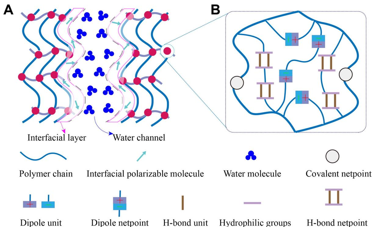
**Figure 1.** (A) Schematic of the PAN-based hydrogel network structure. (B) A typical polymer structural unit with the well-crossed PAN-based hydrogels, including the dual-physical interactions of dipole-dipole pairs and hydrogen bonds, as well as the covalent interaction. PAN: Polyacrylonitrile.
