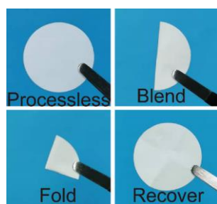
Supplementary Figure 4. Mechanical abuse tests for PEI-EDA separator.
