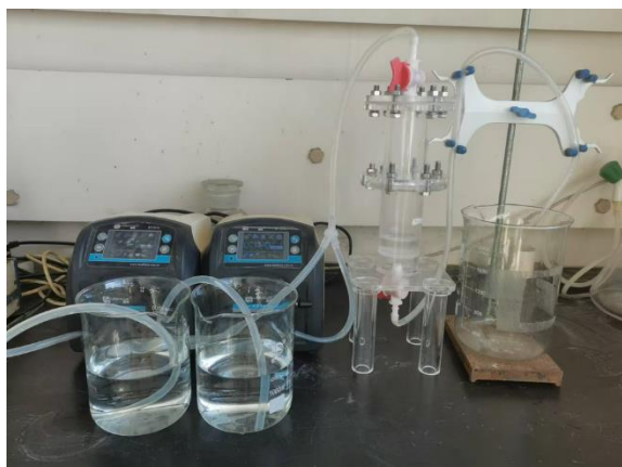
Supplementary Figure 9. Optical photographs of the practical device flow diagram in the dynamic degradation experiment.
