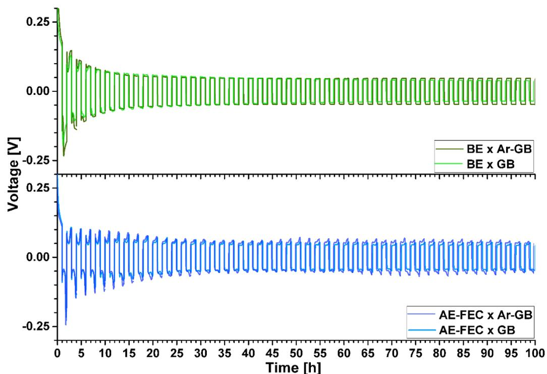
**Supplementary Figure 5.** Close up (100 h/ 50 cycles) of voltage profiles ( $0.5 \text{ mA cm}^{-2}$ , 1 h charge and discharge) of four different Li||Li cell setups comparing ultra-pure  $N_2$  free and “standard” argon glovebox atmosphere (Ar-GB). Top: BE×Ar-GB – dark green, BE×GB – light green; Bottom: AE-FEC×Ar-GB – blue; AE-FEC×GB – light blue.
