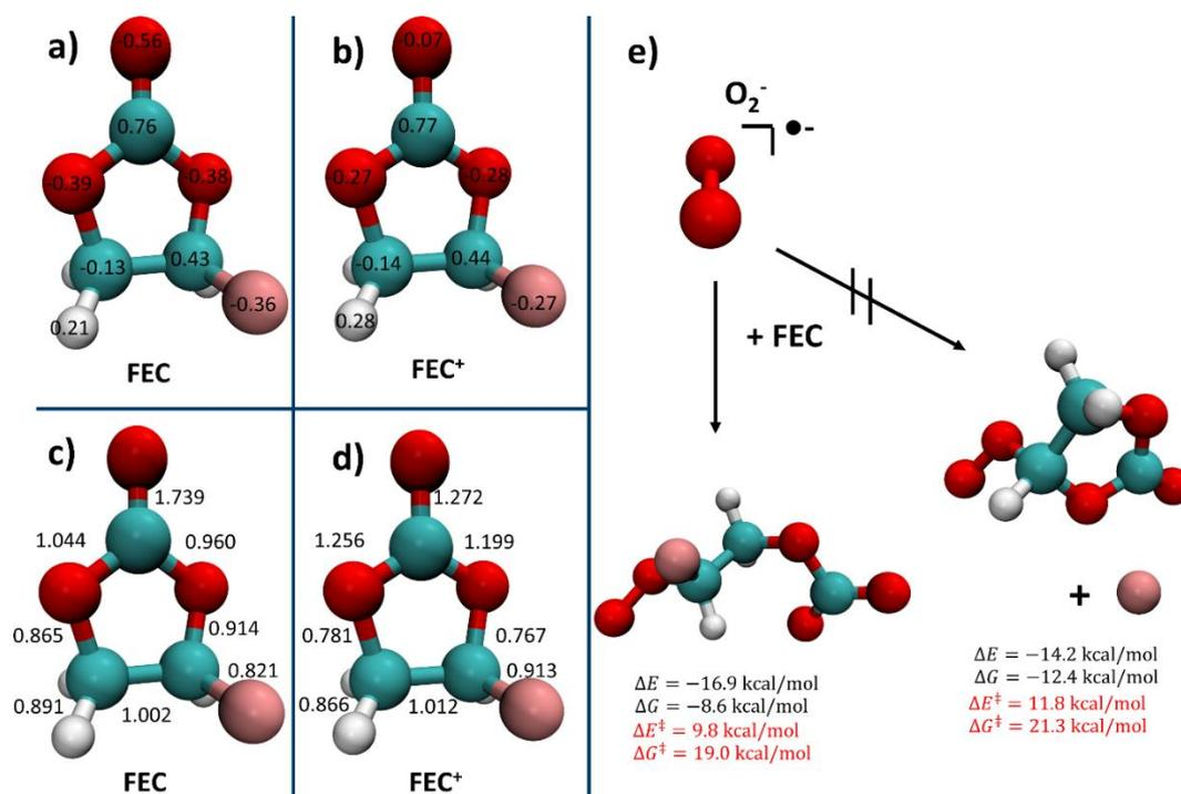
**Supplementary Figure 9.** Quantum chemical calculations as basis for the FEC decomposition mechanism on NMC811 in the presence of oxygen. Mulliken charges (a,b) and bond orders (c,d) of FEC (a, c) and FEC<sup>+</sup> (b, d, representing coordinated an FEC-Li<sup>+</sup> system). E) Free energy (black) and energy barrier (red) values for the nucleophilic attack of the superoxide radical on FEC, supporting a ring opening mechanism over a fluorine cleavage.
