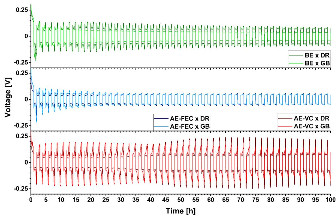
**Supplementary Figure 4.** Close up (100 h/ 50 cycles) of voltage profiles ( $0.5 \text{ mA cm}^{-2}$ , 1 h charge and discharge) of six different Li||Li cell setups. Top: BE×DR – dark green, BE×GB – light green; Middle: AE-FEC×DR – dark blue; AE-FEC×GB – light blue; Bottom: AE-VC×DR – dark red; AE-VC×GB – light red.
