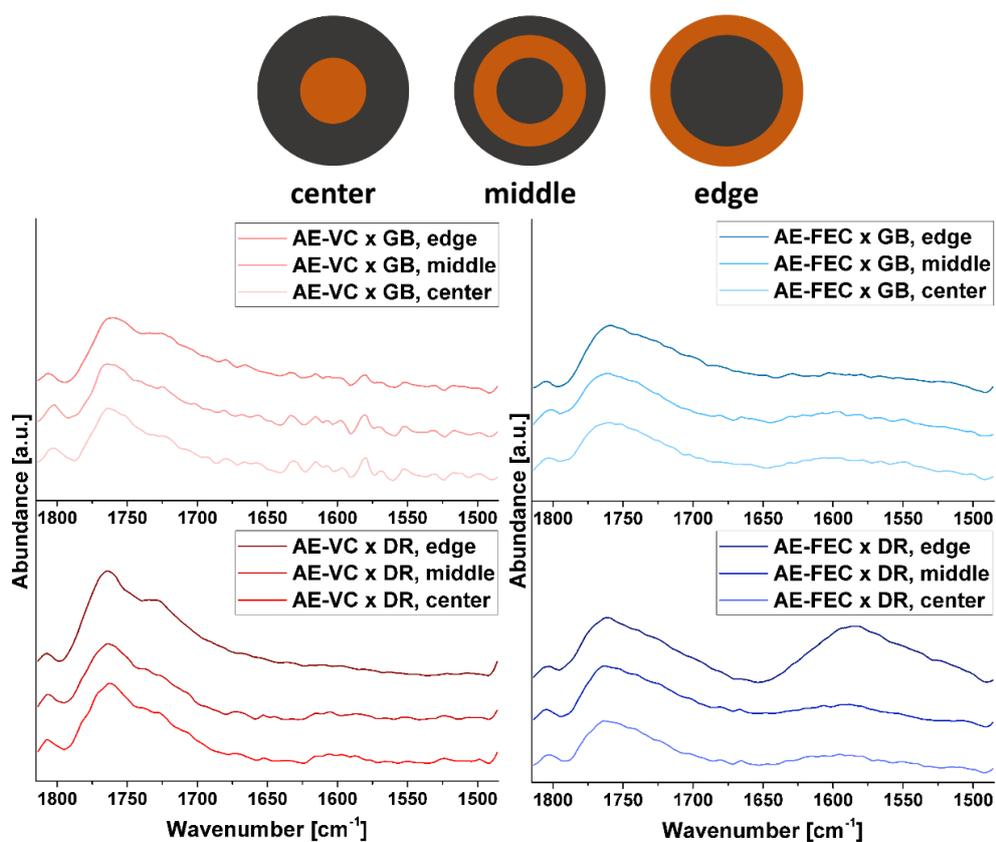
**Supplementary Figure 3.** Additional ATR-FTIR spectra measured on different parts of the electrode (highlighted in orange).
