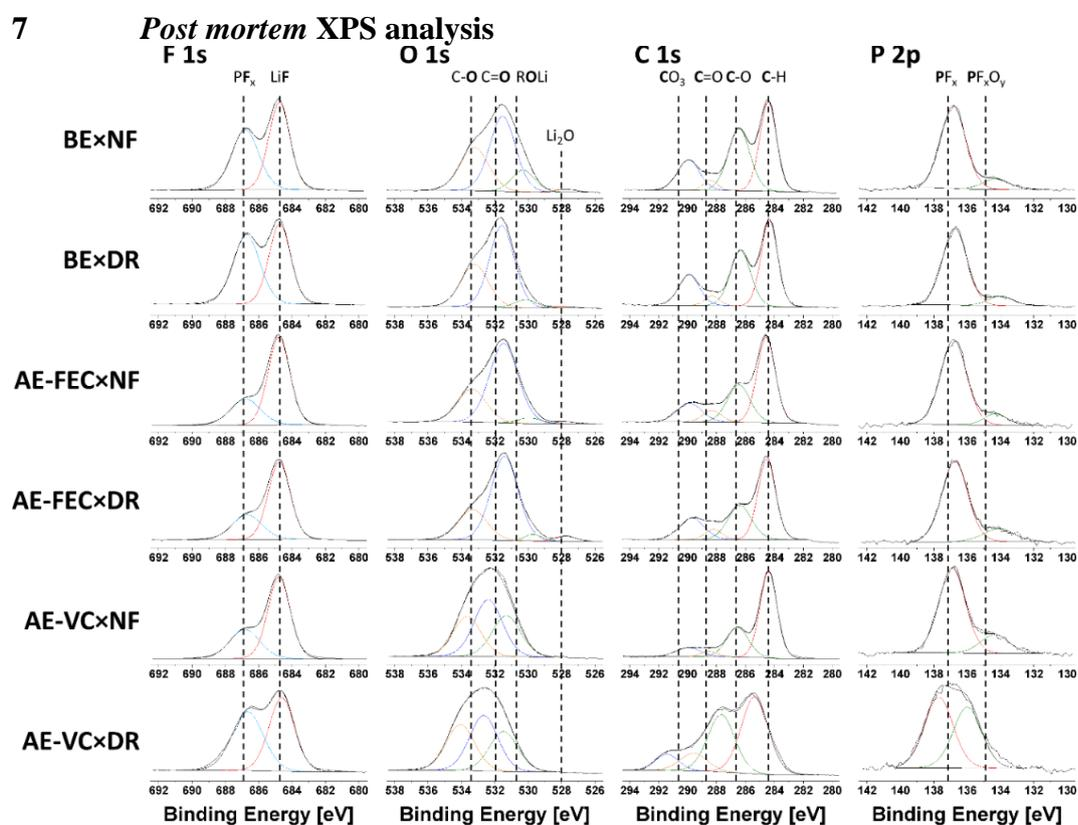
**Supplementary Figure 8.** Individual chemical resonance of the *post mortem* XPS analysis of Li electrodes harvested from Li | Li symmetric cells after 100 h of stripping/plating experiment ( $0.5 \text{ mA cm}^{-2}$ ,  $0.5 \text{ mAh cm}^{-2}$ ).
