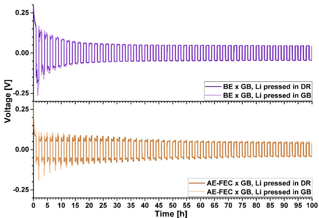
**Supplementary Figure 6.** Close up (100 h/ 50 cycles) voltage profiles ( $0.5 \text{ mA cm}^{-2}$ , 1 h charge and discharge) of four different Li||Li cell setups assembled using either lithium electrodes prepared in a GB or DR atmosphere.[7,39] Top: BE×GB, Li pressed in DR – dark purple, BE×GB, Li pressed in GB – light purple; Bottom: AE-FEC×GB, Li pressed in DR – dark brown; AE-FEC×GB – light brown.
