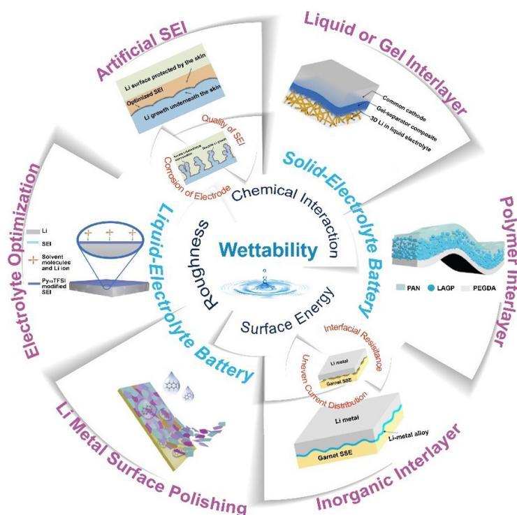
**Figure 1.** Schematic diagram illustrating the lithiophilicity-related studies in rechargeable Li-metal batteries with both liquid and solid electrolytes. Reproduced with permission from Ref. [23] (Copyright 2017, American Association for the Advancement of Science), Ref. [26] (Copyright 2016, Wiley-VCH), Ref. [36] (Copyright 2017, American Chemical Society), Ref. [45] (Copyright 2018, Elsevier), Ref. [64] (Copyright 2019, Wiley-VCH) and Ref. [72] (Copyright 2019, Wiley-VCH).
