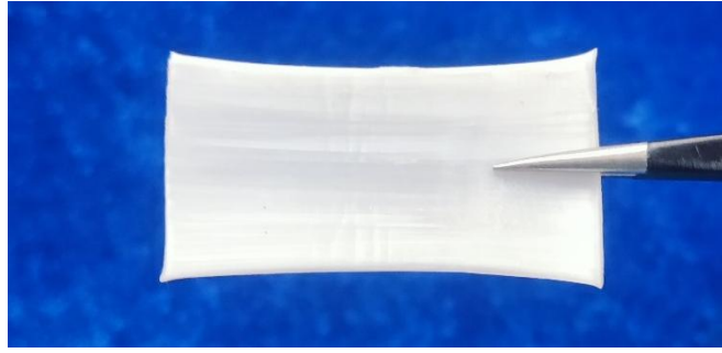
Supplementary Figure 1. Digital image of DFS PVA hydrogel with the stretching ratio of 4.
