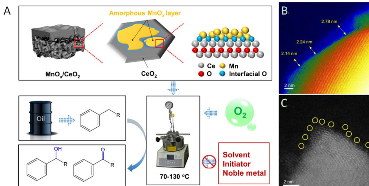
**Figure 1.** (A) Synthetic and catalytic strategies of the ceria-supported two-dimensional manganese oxide catalyst with SOSIs. (B,C) High-resolution STEM images of  $\text{MnO}_x/\text{CeO}_2$  catalyst with SOSIs. The isolated Ce sites in the amorphous region were highlighted by yellow circles in (C)<sup>[6]</sup>.
