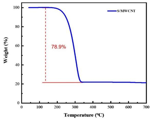
**Supplementary Figure 2.** TGA curves that were recorded for the S/MWCNT.
