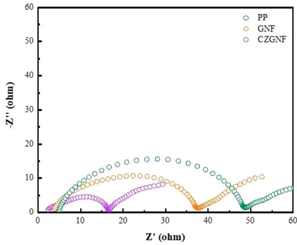
**Supplementary Figure 1.** EIS spectra of Li-S batteries containing the different separators after 100 h.
