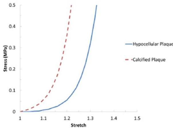
Figure 5. Stress-stretch curve for hypo-cellular and calcified plaque<sup>[13]</sup>
