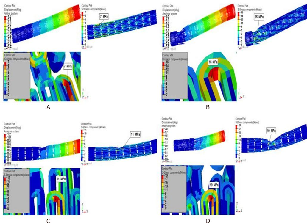
**Figure 3.** Von-mises stress distribution of PEEK 450G stent when subjected to (A) 1 mm displacement (B) 2 mm displacement with 0.1 radian rotation (C) 0.15 radian rotations, (D) 0.25 radian rotations. PEEK: polyether ether ketone
