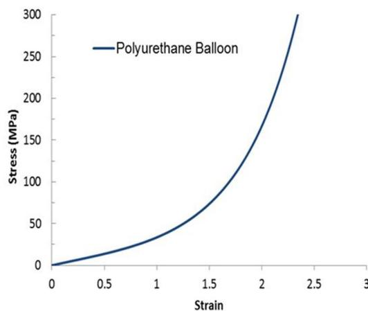
Figure 6. Stress-strain curve for polyurethane rubber balloon<sup>[13]</sup>
