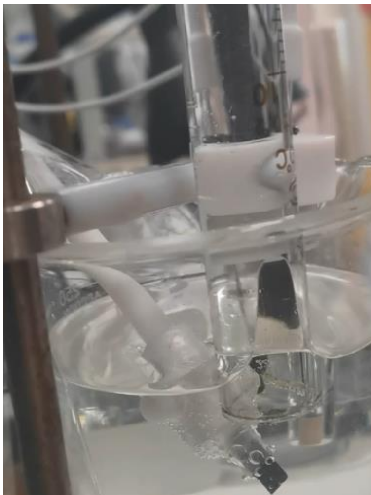
Supplementary Figure 9. The digital photograph captures the hydrogen generated by water drainage strategy.
