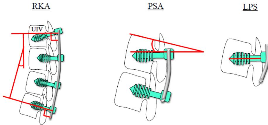
**Figure 3.** Implant-related parameters. RKA: Rod kyphotic angle in the upper instrumented vertebra (UIV)-L1; PSA: pedicle screw angle (angle between the pedicle screw and cranial endplate in the UIV); LPS: length of the UIV pedicle screw; UIV: upper instrumented vertebra.
