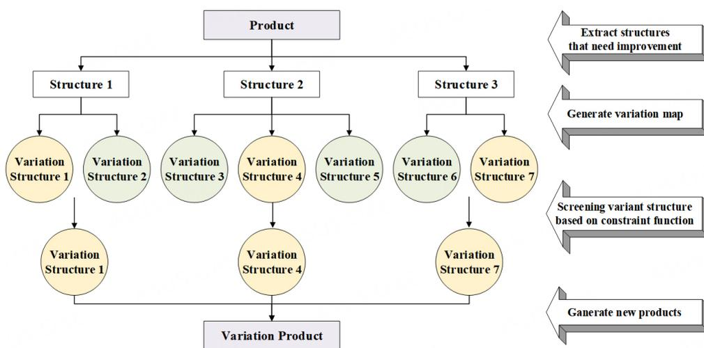
**Figure 3. Schematic diagram of structural variation map generation.**
