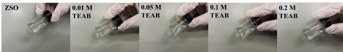
Figure 1. Digital photos of ZSO electrolytes with and without different concentrations of TEAB additives (0, 0.01, 0.05, 0.1 and 0.2 M).
