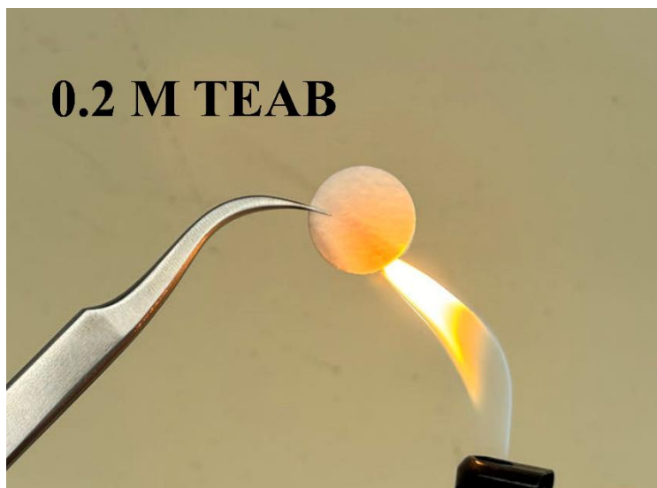
Figure 2. The ignition test of ZSO electrolyte with 0.2 M TEAB additive.
