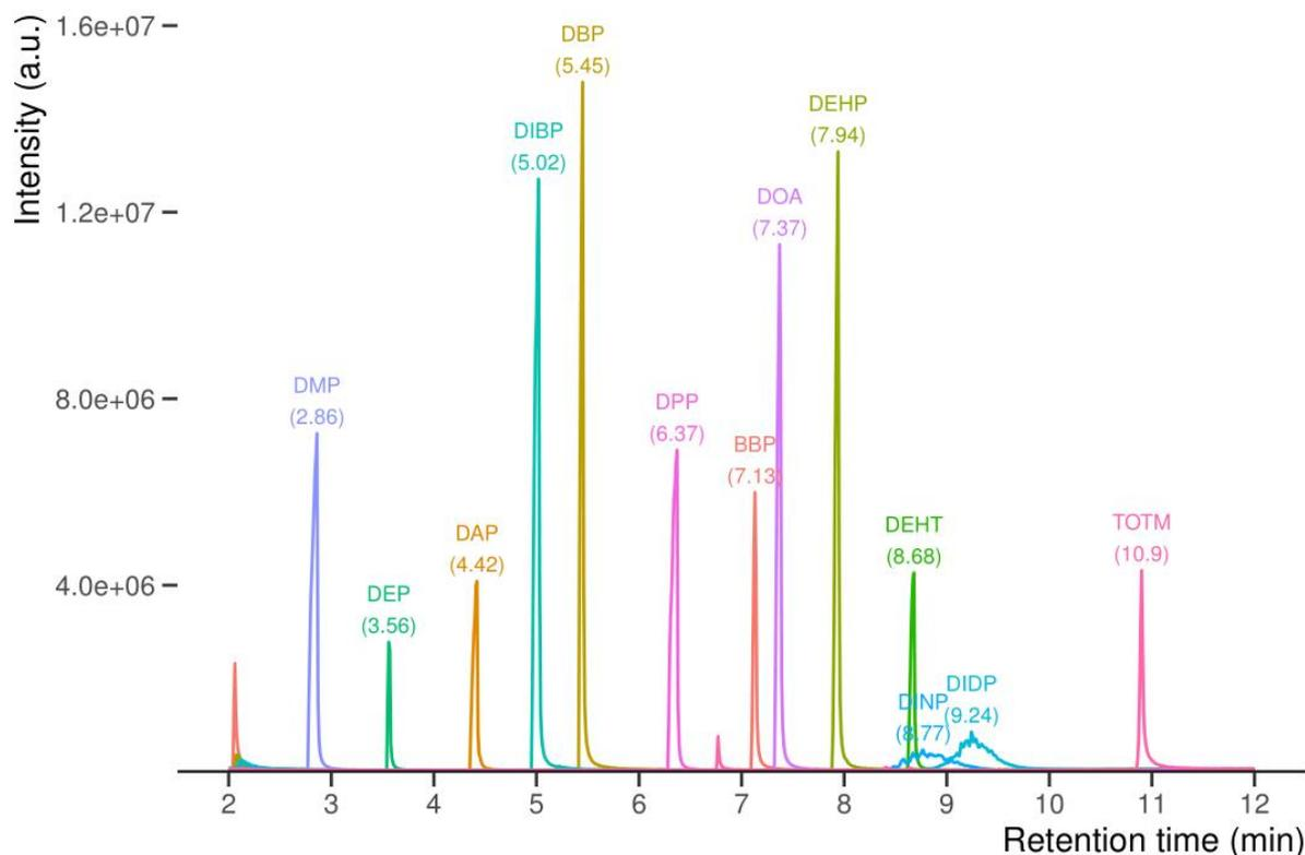
**Figure 2.** Py/TD-GC-MS total ion current chromatograms (SIM mode, overlaid, without normalization) from reference plasticized PVC samples, each with 30% of designated plasticizer and 70% virgin PVC resin.
