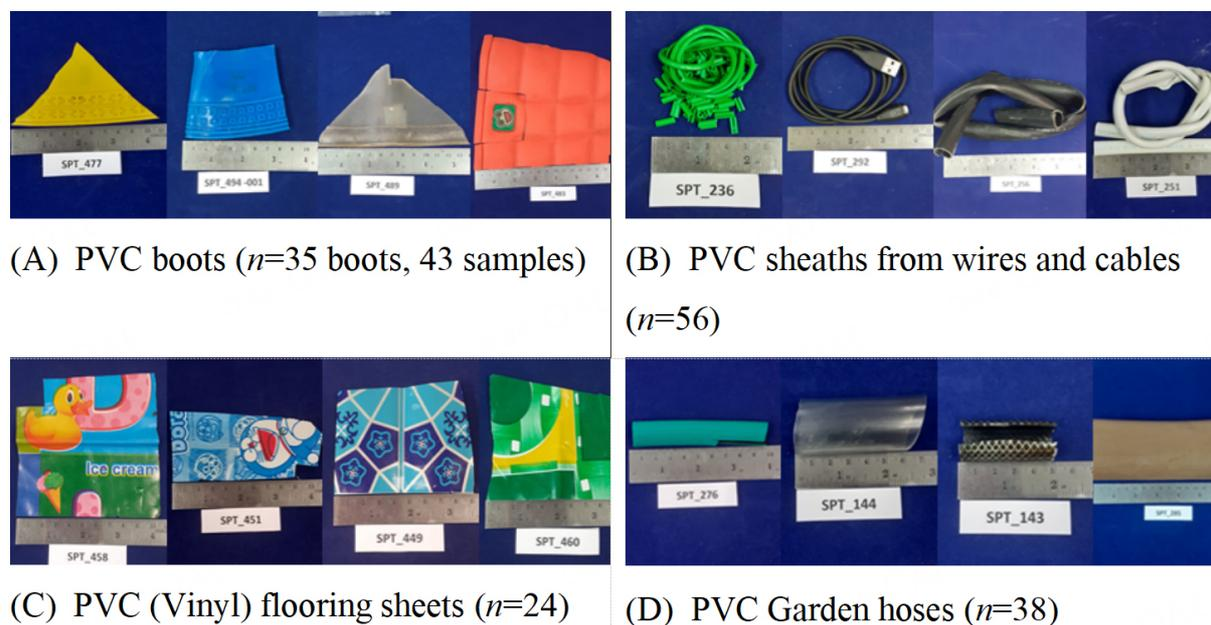
**Figure 1.** Flexible PVC samples analyzed in this study
