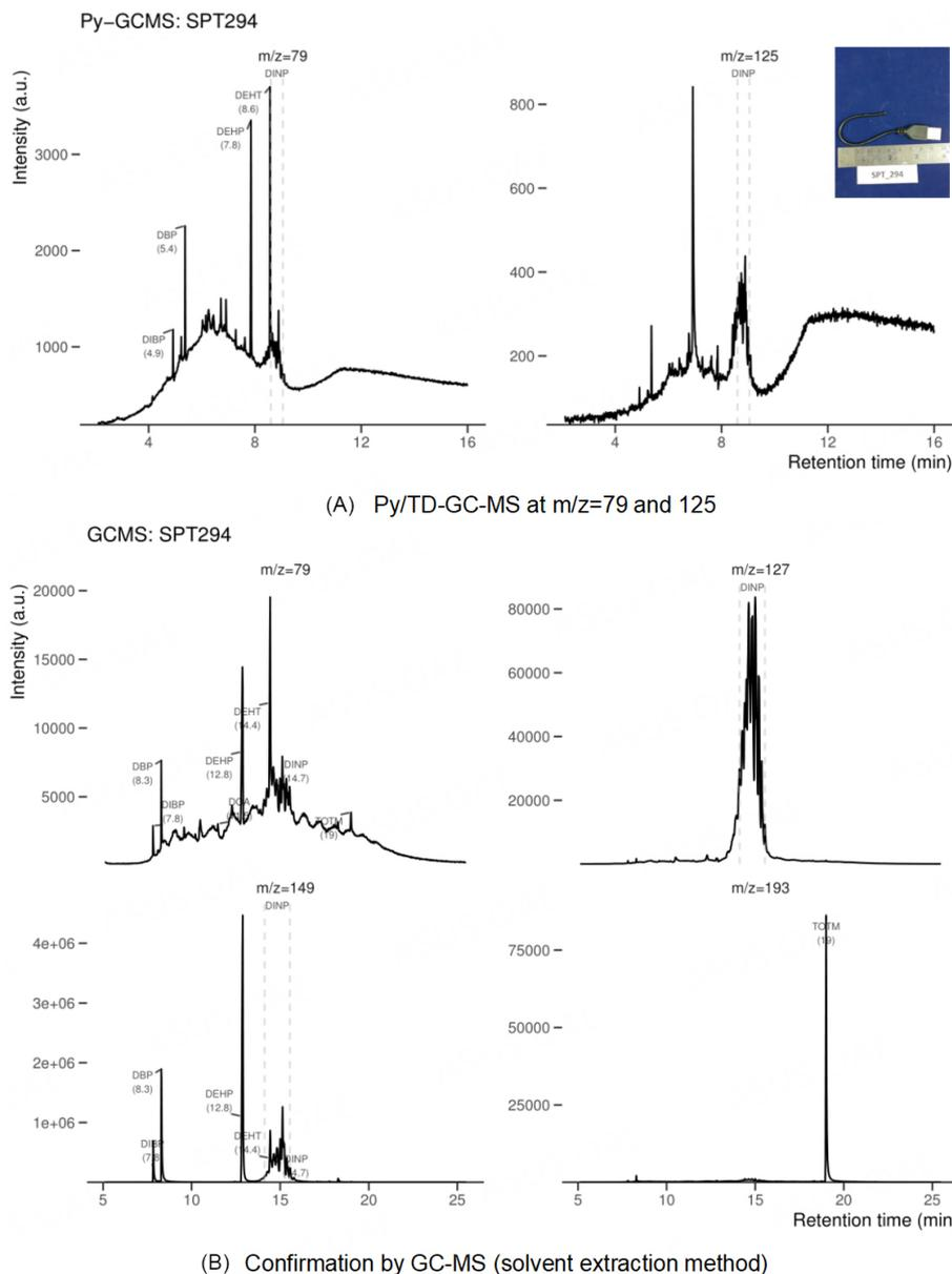
**Figure 4.** Demonstration of (A) Py/TD-GC-MS chromatograms (SIM mode,  $m/z$  79 and 125) from a sample (cable); and (B) the corresponding GC-MS chromatograms (SIM Mode,  $m/z$  79, 127, 149 and 193) from solvent extraction method.
