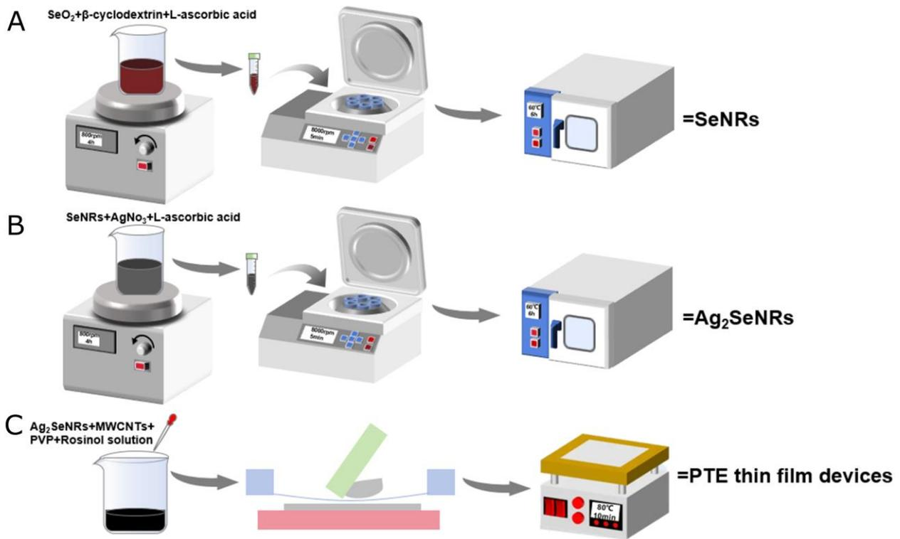
**Supplementary Figure 1.** (A) SeNRs preparation method; (B)  $\text{Ag}_2\text{Se}$  NRs preparation method; (C) PTE detector preparation method.
