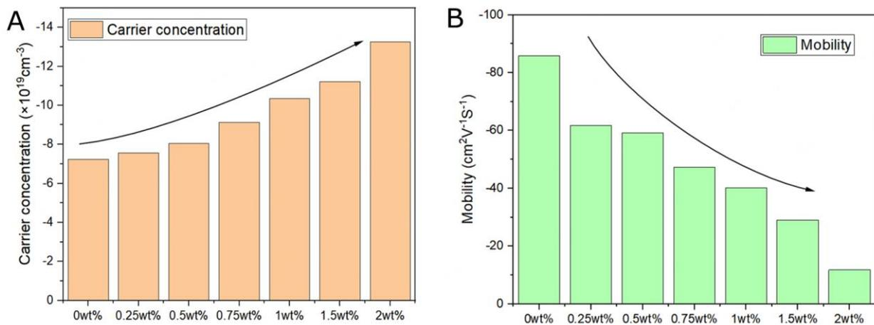
**Supplementary Figure 2.** (A) Variation of carrier concentration with MWCNTs content; (B) Variation of mobility with MWCNTs content.
