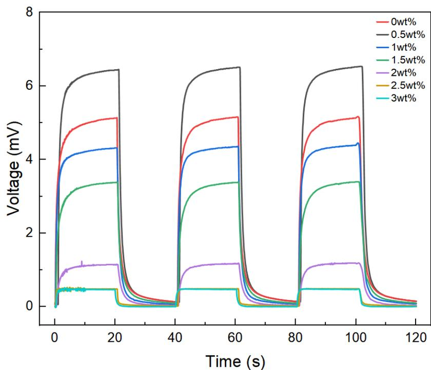
**Supplementary Figure 4.** PTE output voltage curves for MWCNTs from 0-3 wt% at 650 nm 100 mW laser.
