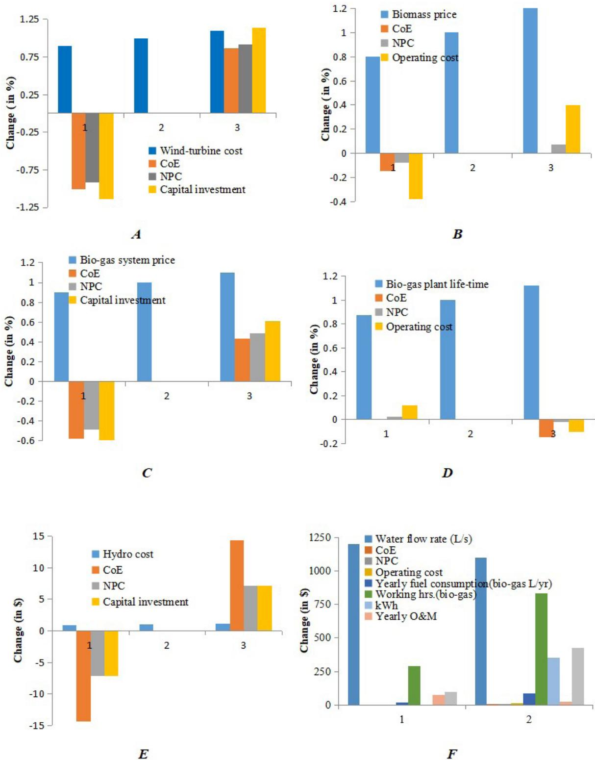
**Figure 5.** Sensitivity analysis for (A) wind-turbine price; (B) biomass price; (C) bio-gas genset system price; (D) bio-gas system life; (E) hydropower system cost; and (F) water flow rate for hydro-power.
