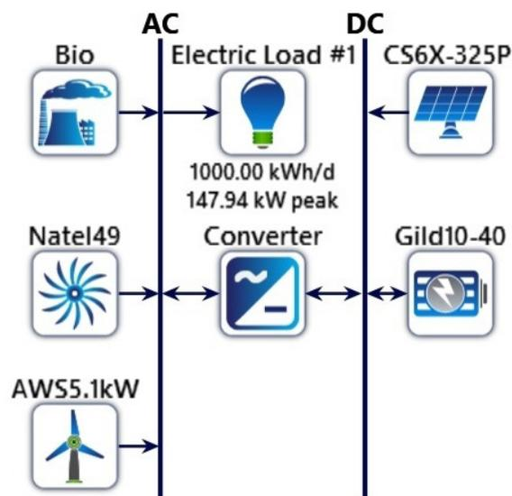
**Figure 1.** The microgrid power system model for Arusha, Tanzania developed in HOMER Pro<sup>[39]</sup>.
