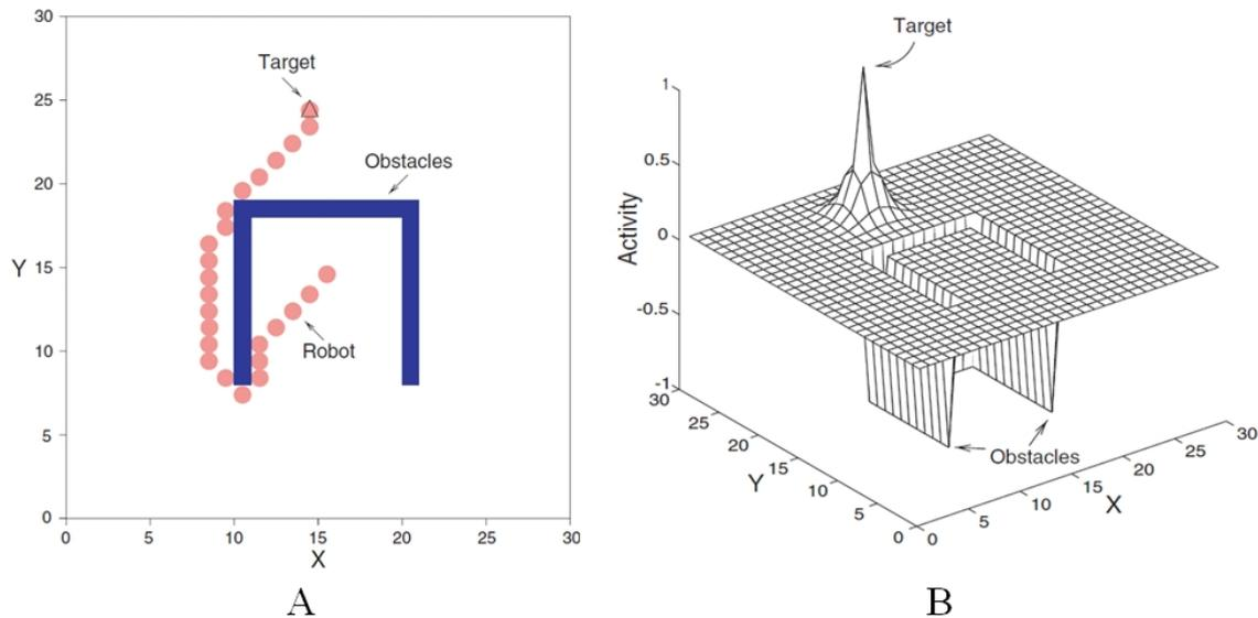
**Figure 4.** Path planning of a mobile robot to avoid local minima with concave obstacles. A: the robot path; B: the landscape of neural activity<sup>[13]</sup>.
