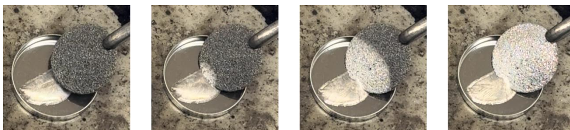
Supplementary Figure 4. Digital photos of molten Li infusion in NF-CNT500.
