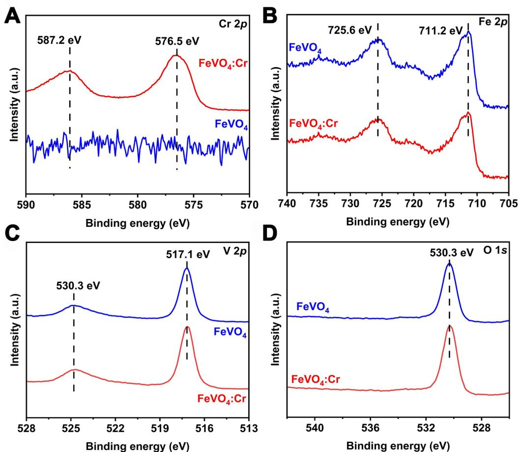
**Supplementary Figure 11.** X-ray photoelectron spectroscopy (XPS) (A) Cr 2p, (B) Fe 2p, (C) V 2p and (D) O 1s of FeVO<sub>4</sub> and FeVO<sub>4</sub>:Cr samples.
