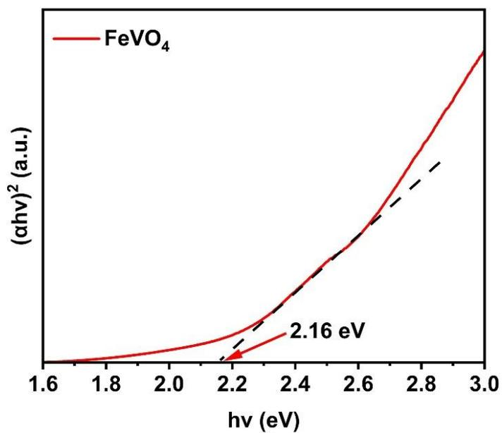
Supplementary Figure 4. Tauc plot of FeVO<sub>4</sub> (obtained from Figure 1A).
