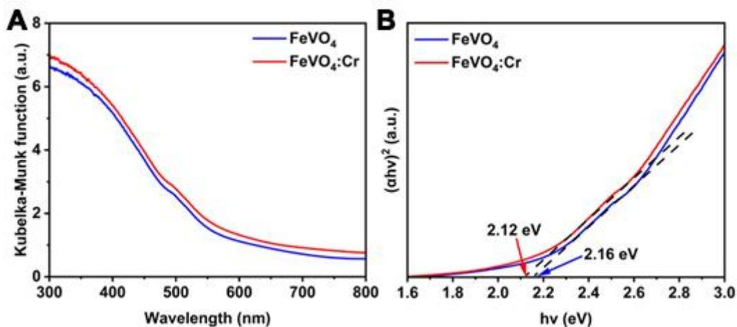
**Supplementary Figure 10.** (A) The ultraviolet-visible diffuse reflectance spectra obtained using Kubelka-Munk function and (B) Tauc plots of FeVO<sub>4</sub> and FeVO<sub>4</sub>:Cr samples.
