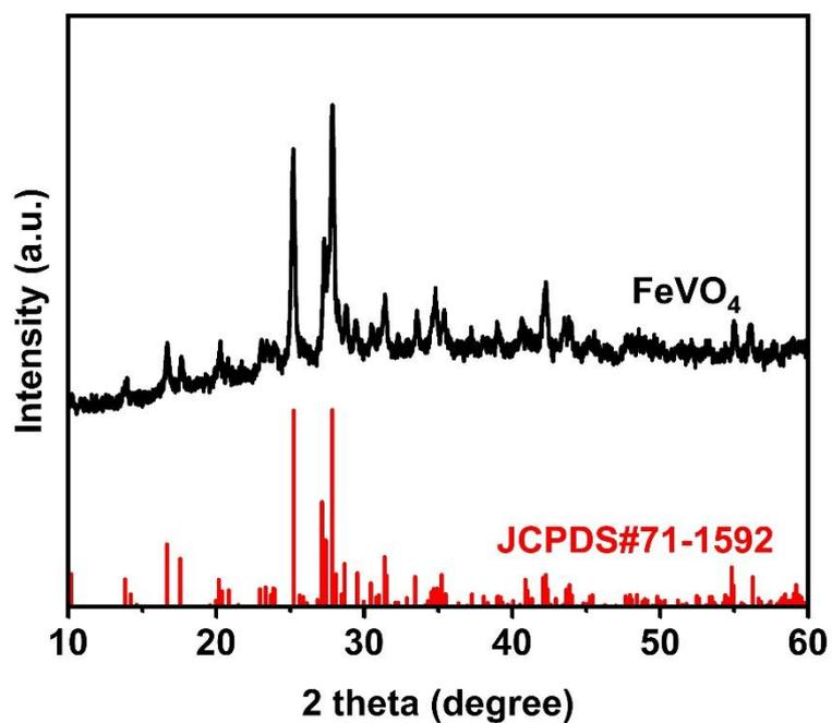
**Supplementary Figure 1.** X-Ray diffraction (XRD) pattern of FeVO<sub>4</sub>.
