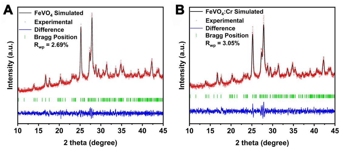
**Supplementary Figure 8.** Rietveld refined XRD patterns of (A) FeVO<sub>4</sub> and (B) FeVO<sub>4</sub>:Cr samples.
