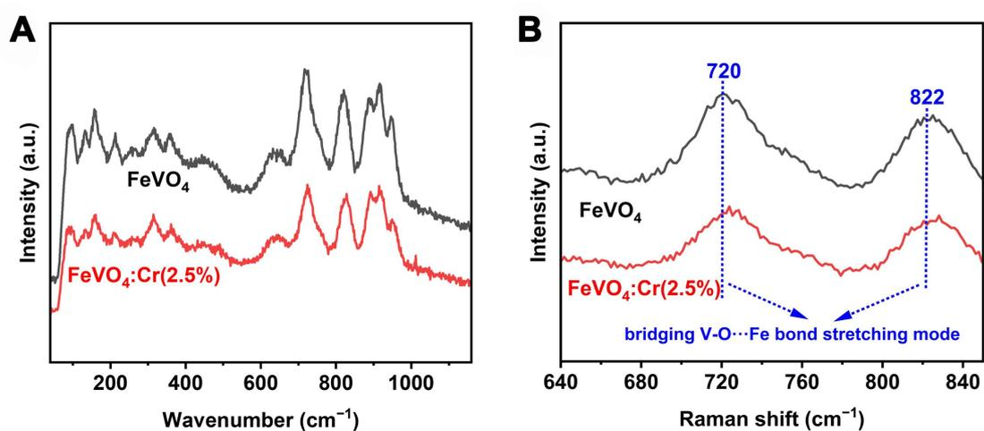
**Supplementary Figure 9.** (A) Raman spectra and (B) enlarged Raman spectra of FeVO<sub>4</sub> and FeVO<sub>4</sub>:Cr samples.
