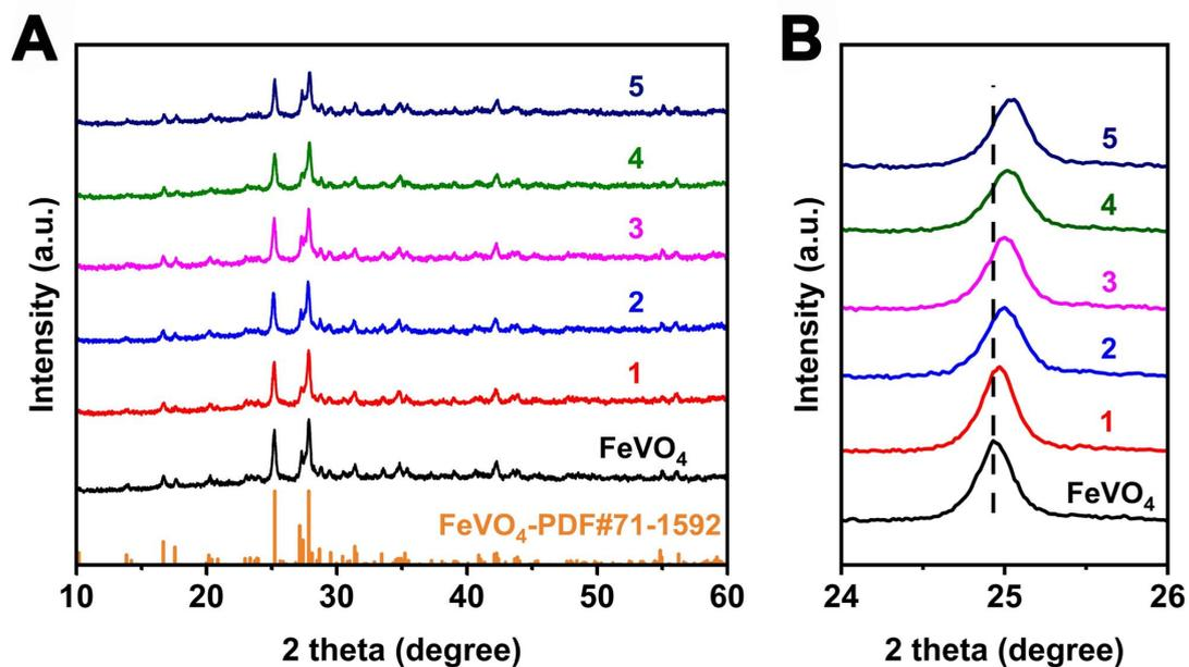
**Supplementary Figure 7.** (A) XRD patterns and (B) enlarged XRD patterns of FeVO<sub>4</sub>:Cr samples with different doping proportions. Herein, 1: FeVO<sub>4</sub>:Cr(1.5%), 2: FeVO<sub>4</sub>:Cr(2.0%), 3: FeVO<sub>4</sub>:Cr(2.5%), 4: FeVO<sub>4</sub>:Cr(3.0%), 5: FeVO<sub>4</sub>:Cr(3.5%).
