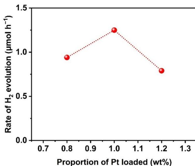
**Supplementary Figure 13.** Effect of the loaded proportion of Pt on the initial H<sub>2</sub> evolution rate over Pt/FeVO<sub>4</sub>:Cr sample (the molar ratio of Cr/(Cr+Fe) is 3%). Reaction conditions: 0.1 g of photocatalyst; 100 mL of ascorbic acid aqueous solution (10 mM); 300 W Xe lamp with a cutoff filter ( $\lambda \geq 420$  nm).
