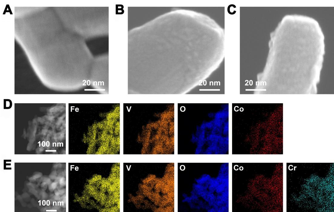
**Supplementary Figure 16.** SEM images of (A) FeVO<sub>4</sub>, (B) CoO<sub>x</sub>/FeVO<sub>4</sub> and (C) CoO<sub>x</sub>/FeVO<sub>4</sub>:Cr samples. EDS mapping images of (D) CoO<sub>x</sub>/FeVO<sub>4</sub> and (E) CoO<sub>x</sub>/FeVO<sub>4</sub>:Cr samples.
