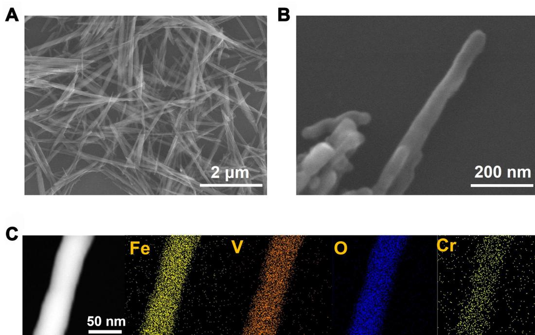
**Supplementary Figure 5.** SEM images of (A) FeVO<sub>4</sub>:Cr·1.1H<sub>2</sub>O and (B) FeVO<sub>4</sub>:Cr samples. (C) Energy dispersive X-ray spectroscopy (EDS) mapping images of FeVO<sub>4</sub>:Cr sample.
