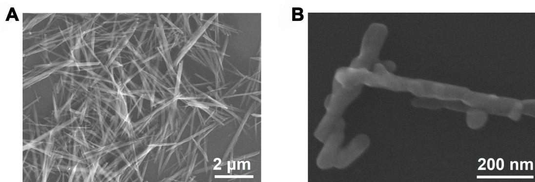
**Supplementary Figure 2.** Scanning electron microscope (SEM) images of (A) FeVO<sub>4</sub>·1.1H<sub>2</sub>O and (B) FeVO<sub>4</sub>.
