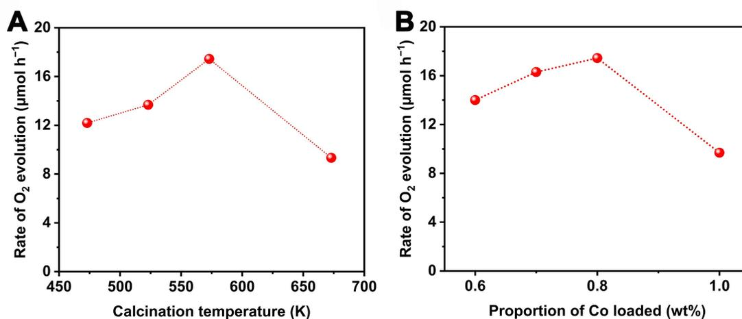
**Supplementary Figure 12.** Effect of (A) the calcination temperature and (B) the loaded proportion of CoO<sub>x</sub> on the initial O<sub>2</sub> evolution rate over CoO<sub>x</sub>/FeVO<sub>4</sub>:Cr sample (the molar ratio of Cr/(Cr+Fe) is 2.5%). Reaction conditions: 0.1 g of photocatalyst; 100 mL of AgNO<sub>3</sub> aqueous solution (50 mM); 0.1 g of La<sub>2</sub>O<sub>3</sub>; 300 W Xe lamp with a cutoff filter ( $\lambda \geq 420$  nm).
