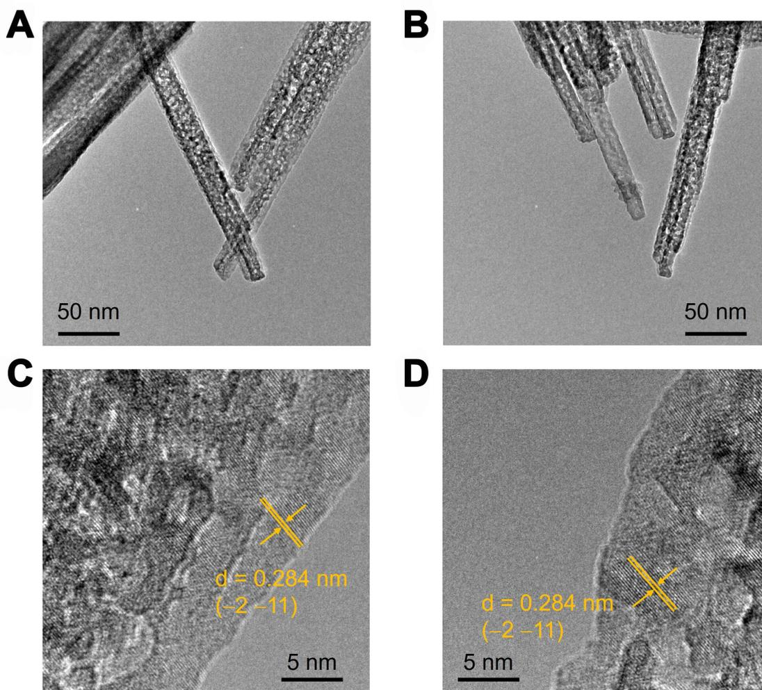
**Supplementary Figure 6.** Transmission electron microscopy (TEM) images of (A) FeVO<sub>4</sub> and (B) FeVO<sub>4</sub>:Cr samples. (C) High-resolution TEM (HRTEM) images of (C) FeVO<sub>4</sub> and (D) FeVO<sub>4</sub>:Cr samples.
