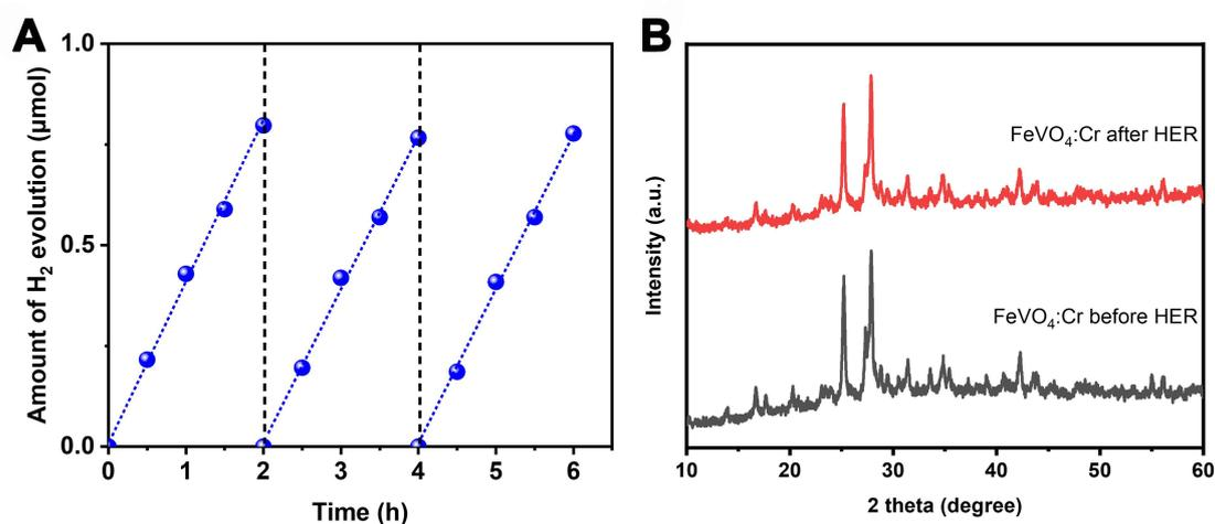
**Supplementary Figure 14.** (A) The recycling test of H<sub>2</sub> generation over FeVO<sub>4</sub>:Cr photocatalyst loaded with Pt cocatalyst. Reaction conditions: 0.1 g of photocatalyst (1.0 wt% Pt is loaded); 100 mL of ascorbic acid aqueous solution (10 mM); 300 W Xe lamp with a cutoff filter ( $\lambda \geq 420$  nm). (B) XRD patterns of FeVO<sub>4</sub>:Cr samples before and after the HER (hydrogen evolution reaction). The molar ratio of Cr/(Cr+Fe) in FeVO<sub>4</sub>:Cr is 3%.
