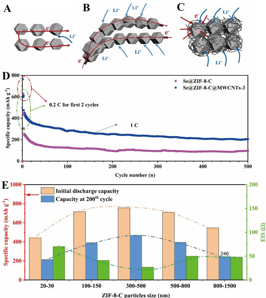
**Figure 1.** Schematic mechanism of the (A) Se@ZIF-8-C, (B) ZIF-8-C@MWCNTs-1 and (C) Se@ZIF-8-C@MWCNTs-5 electrodes for lithium ion and electron movement. (D) Cycling performance of Se@ZIF-8-C and Se@ZIF-8-C@MWCNTs-3 at high current density of 1 C, (E) summary of the specific capacity and impedance of the Se@ZIF-8-C@MWCNTs-X (X = 1-5) positive electrodes according to the particle size of the internal ZIF-8 derived porous carbon.
