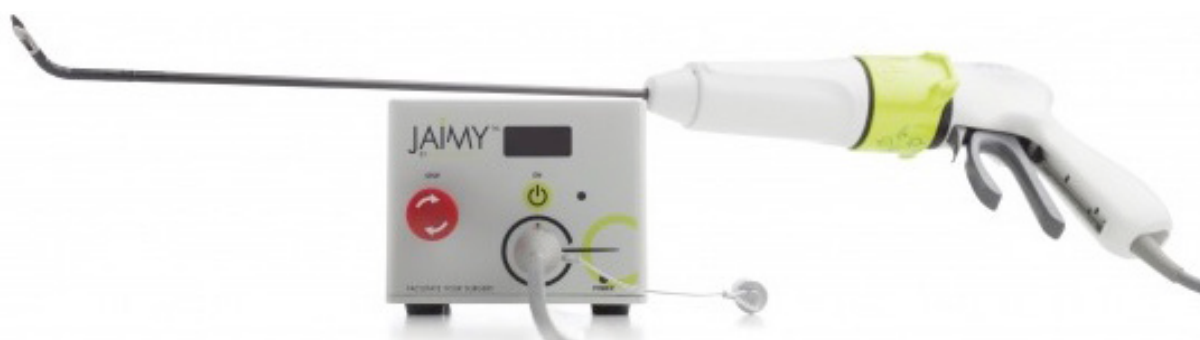
Figure 4. Articulating 5-mm laparoscopic instrument with motorized control (JAIMY-EN, Endocontrol, Grenoble, France)
