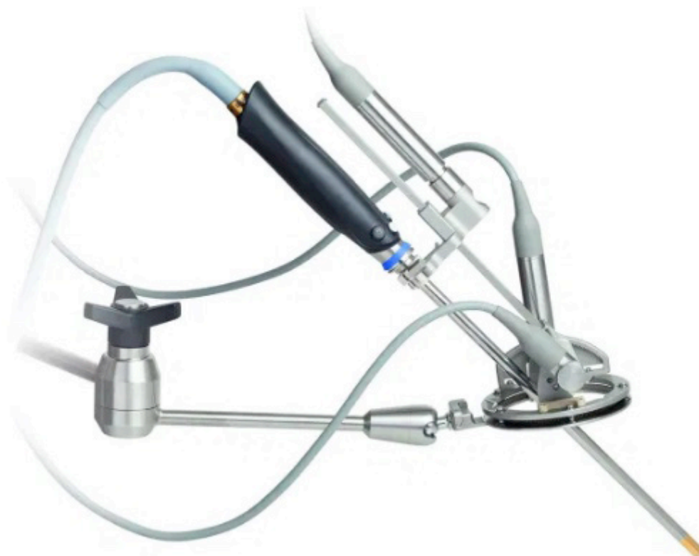
Figure 3. VideoendosKopY (ViKY) robotically-controlled laparoscope holder (ViKY, Endocontrol, Grenoble, France)
