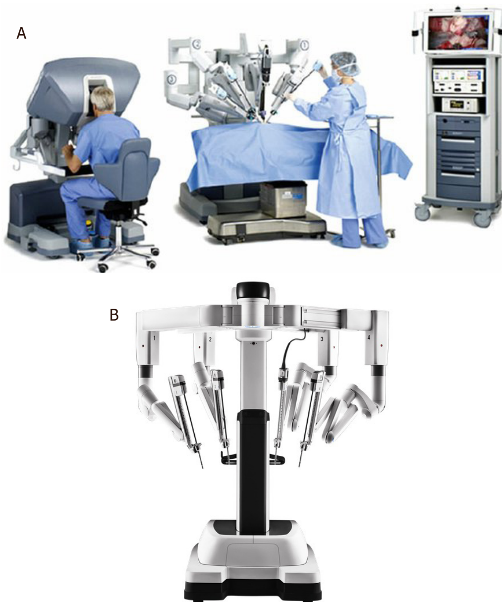
Figure 1. A: da Vinci complete surgical robotic systems have three major components: (1) the surgeon's console; (2) a surgical cart with the robotic arms and end-effectors; and (3) the visual cart (copyright Intuitive Surgical International - reproduced courtesy of the manufacturer); B: the latest iteration of the surgical cart for the da Vinci Xi Surgical System (da Vinci, Intuitive Surgical, Sunnyvale, CA, USA)
