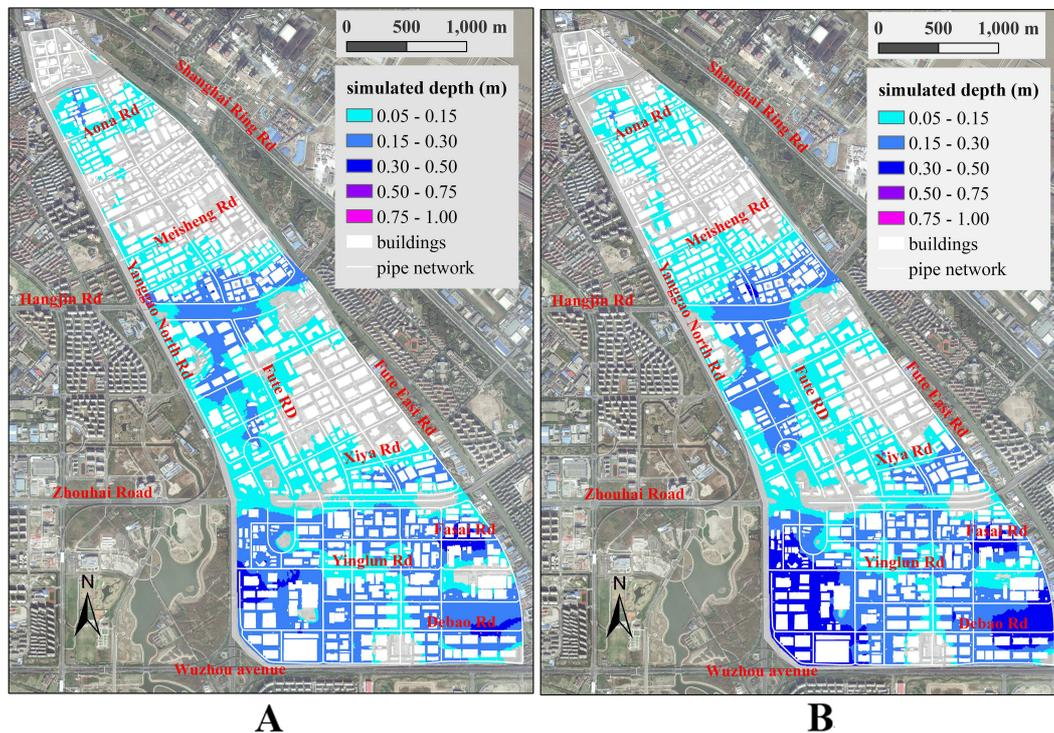
**Figure 5.** Simulated depth distribution of Scenario VII ( $P = 10$  a,  $H = 2.0$  m): (A) surface water depth distribution at  $t = 60$  min; and (B) surface water depth distribution at  $t = 90$  min.
