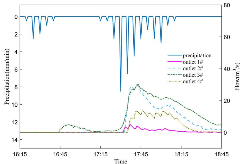
**Figure 3.** Comparison diagram of outlet discharge and precipitation in the study area.
