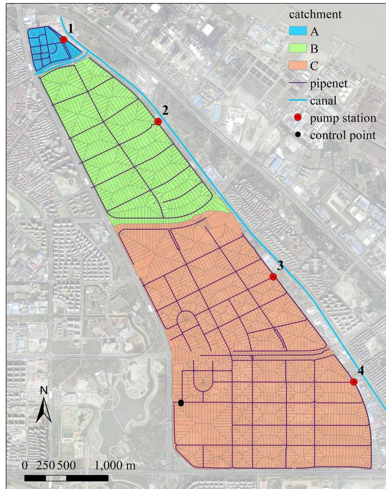
**Figure 2.** Drainage network generalization and catchment division.
