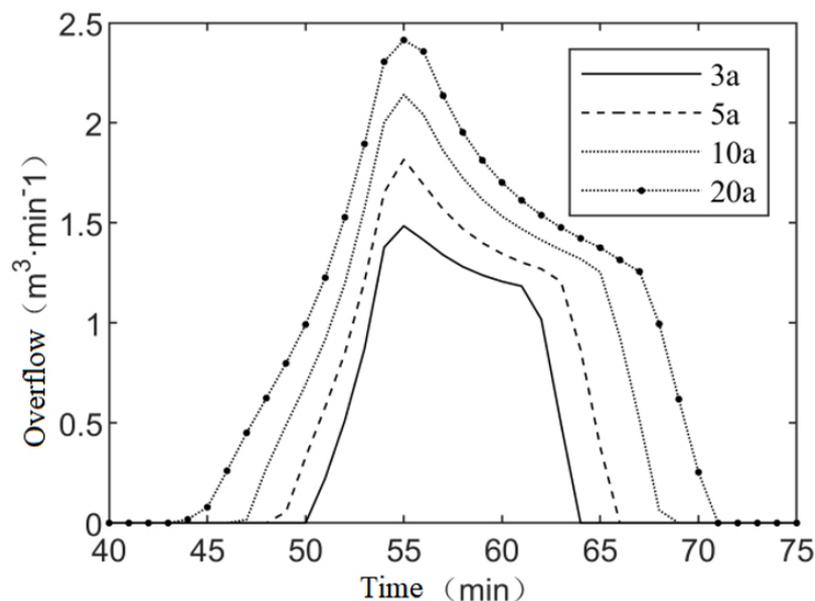
**Figure 7.** Simulated overflow from a typical node under different return periods.
