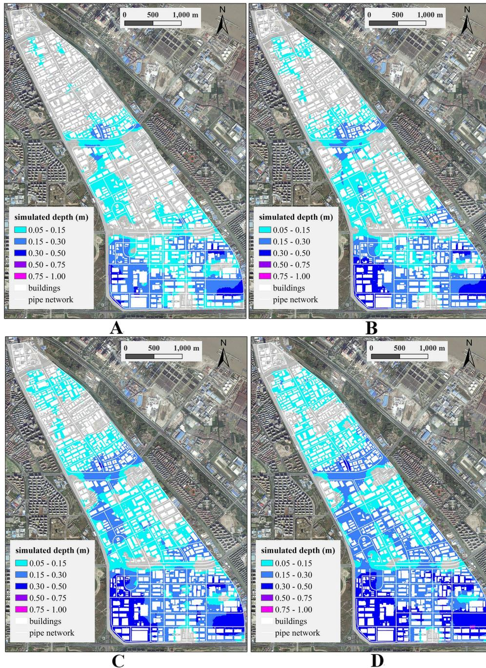
**Figure 6.** Comparison of water depth distribution in different rainfall return periods: (A) water depth distribution of Scenario V ( $P = 3$  a,  $H = 2.0$  m); (B) water depth distribution of Scenario VI ( $P = 5$  a,  $H = 2.0$  m); (C) water depth distribution of Scenario VII ( $P = 10$  a,  $H = 2.0$  m); and (D) water depth distribution of Scenario VIII ( $P = 20$  a,  $H = 2.0$  m).
