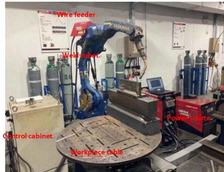
Figure 13. Robot system.
