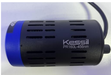
Supplementary Figure 3 Photoreactor used in this research (20 W blue LEDs, \lambda_{\max} = 456 nm)
