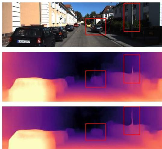
**Figure 1.** The input image from the KITTI dataset (top); the baseline MonoDepth2<sup>[22]</sup> (M, ResNet50, without pre-training) depth prediction; (middle) and our result (bottom).
